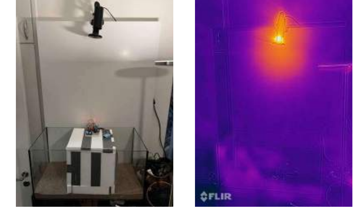
Experimental setup of heat lamp simulating extreme warm heat cycle
